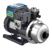
HQ-B is a complete, all-in-one unit, consisting of pump, motor, pressure tank, and electronic controller. The built-in electronic controller provides constant pressure which ensures that the pump starts automatically when water is consumed and operates continuously until water is not required.
