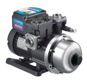
HQCN is a complete, all-in-one unit, consisting of pump, motor, pressure tank, and electronic controller. The built-in electronic controller provides constant pressure which ensures that the pump starts automatically when water is consumed and operates continuously until water is not required.
